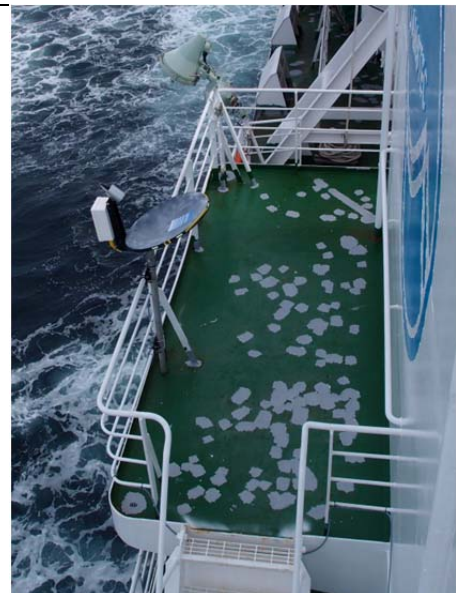
Fig. 2.4-2: The micro rain radar, installed on the starboard side of the anti-rolling tank.
