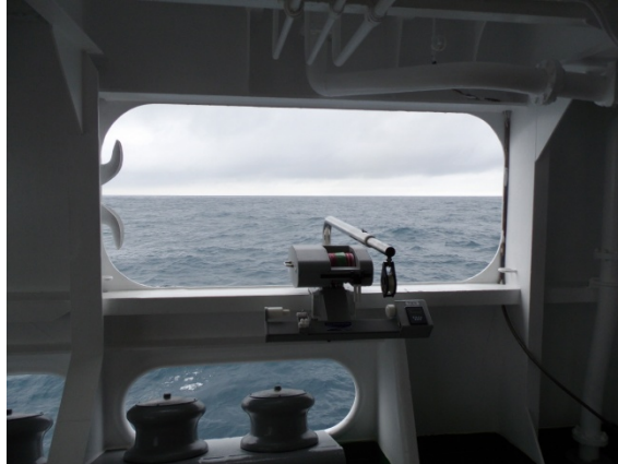
Figure 3.3-1: A whole set of U-CTD system installed on a lower stern deck of R/V Mirai.
