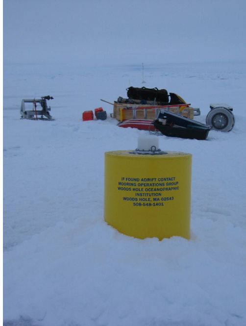
ITP9 (foreground) and IMB (background) with installation apparatus (to be removed from the ice) after deployment from a helicopter supported remote ice camp operation from the Russian research vessel "Akademik Federov". Photo by John Kemp.
