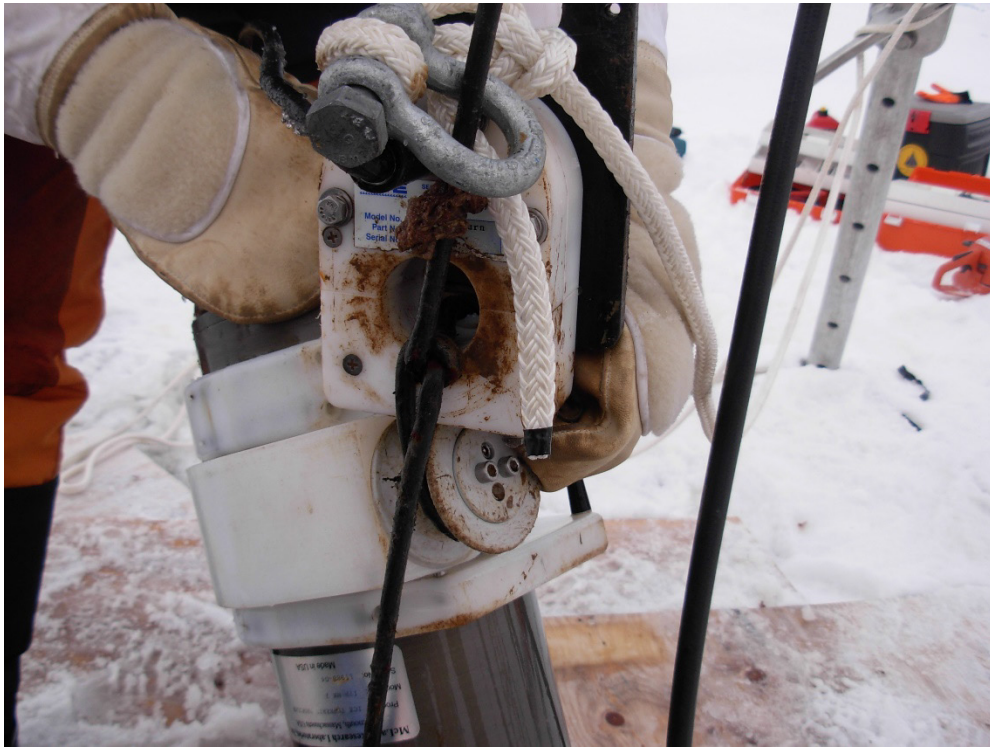
A close-up of the wire tangle around the inductive modem. Surprisingly, despite the snarl, the instrument continued to ring the surface unit after every attempted profile, although a problem with the surface unit modem electronics prevented the transfer of data. Photo by Rick Krishfield.
