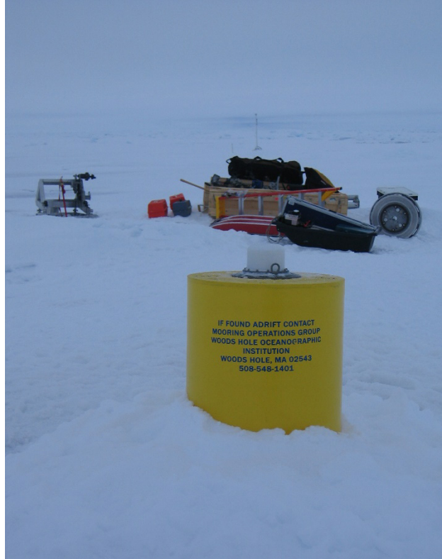
ITP9 (foreground) and IMB (background) with installation apparatus (to be removed from the ice) after deployment from a helicopter supported remote ice camp operation from the Russian research vessel "Akademik Federov". Photo by John Kemp.
