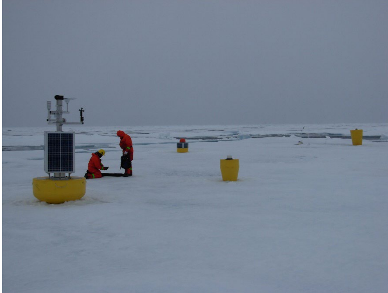
Just prior to returning to the ship, the last crewmembers on the ice pack up the bear protection shortly after the second and last Ice-Based Observatory was deployed during JOIS 2012 consisting of (from left to right), an O-buoy, AOFB, ITM, IMBB, and ITP 66. (Rick Krishfield)
