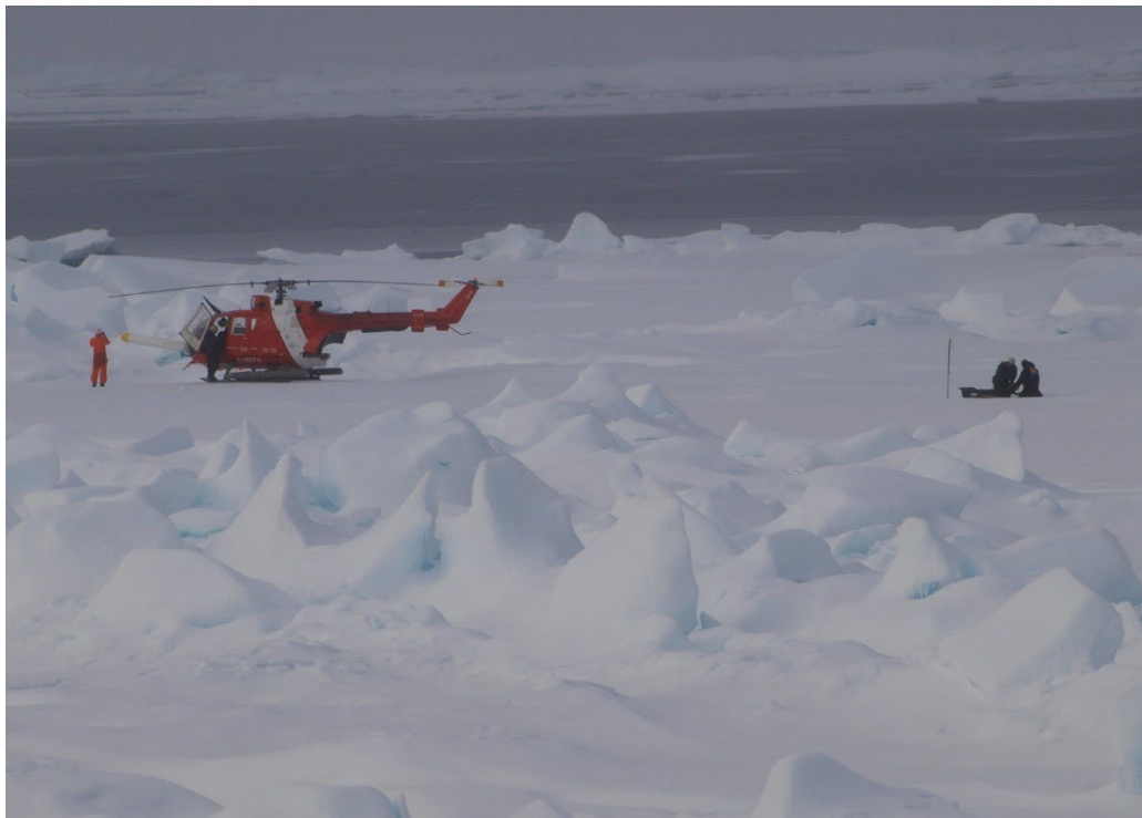
View from the ship of the helicopter landed on the ice while the thickness of the floe is determined at several sites prior to selection of it as the deployment site of the IBO. (Photo by Gary Morgan)
