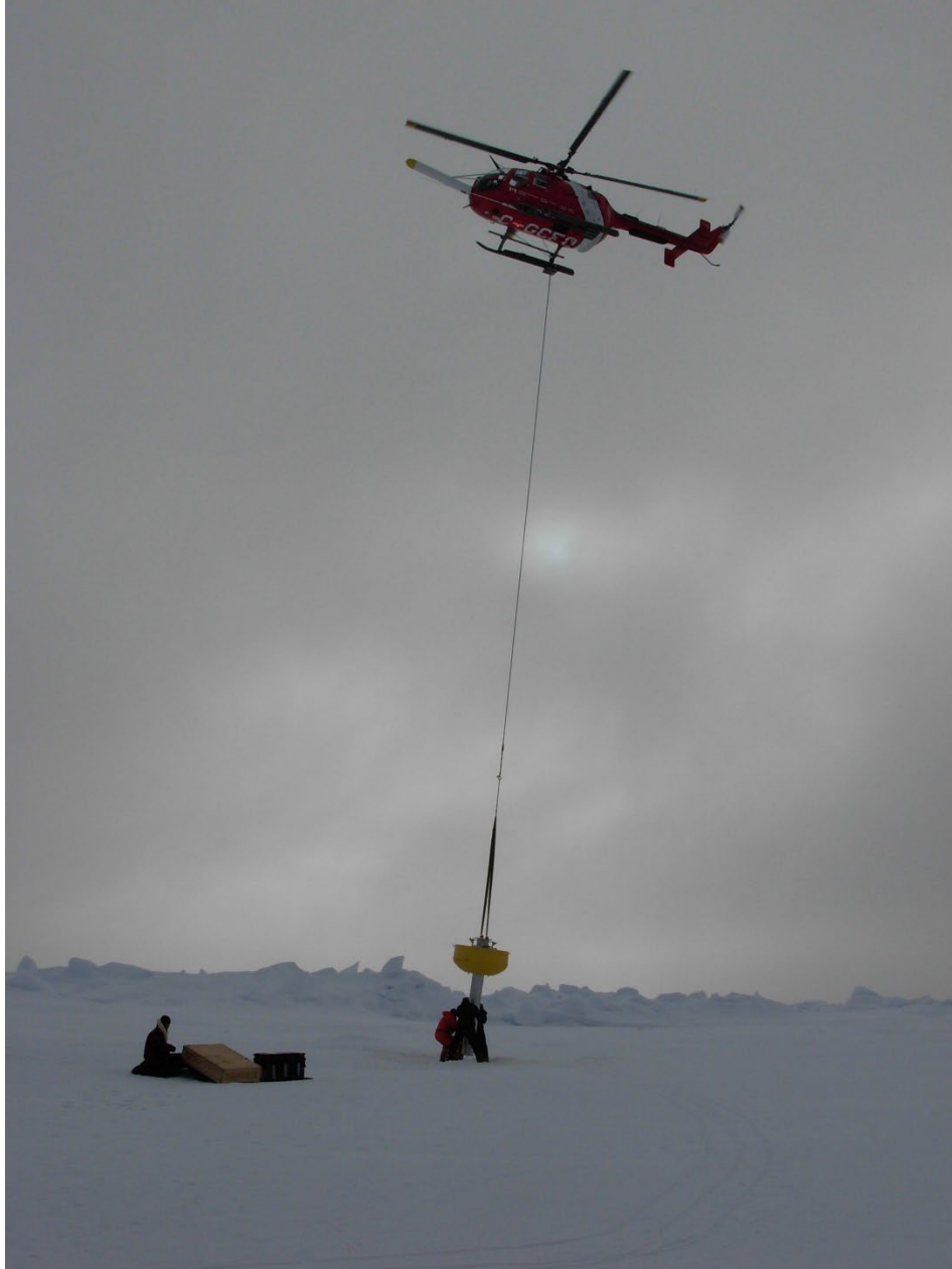
O-Buoy (with superstructure removed) being lowered through the 14" diameter hole in the ice by the helicopter. (Photo by Rick Krishfield)
