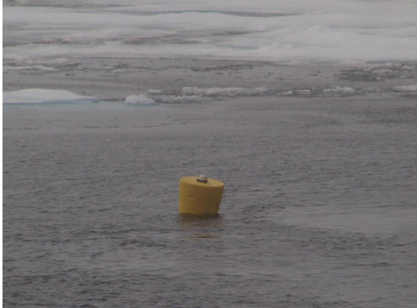
Shortly after being released over-the-side of the ship into open water, ITP 64 waits to be surrounded by the nearby ice floes and frozen into the pack. (Photo by Gary Morgan)
