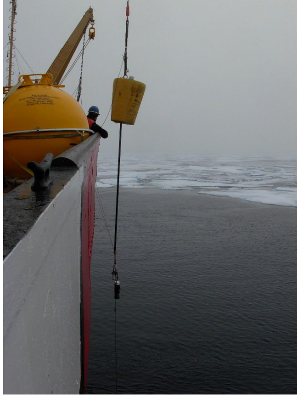
The complete ITP system is lowered into the seawater by the ship's crane. (Photo by Rick Krishfield)
