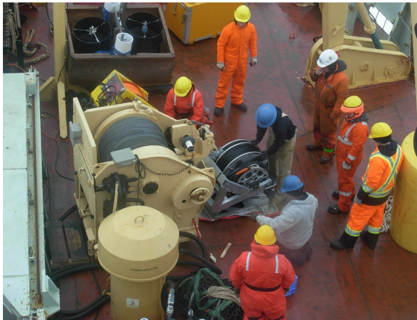
The ITP deployment winch and reel are fastened to the hydro winch on the foredeck for deployment over-the-side. (Photo by Rick Krishfield)
