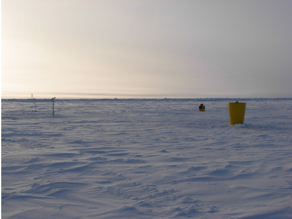
The installed IBO consisting of (from left to right): PAWS, seasonal IMB, AOFB, and ITP 61. (Rick Krishfield)
