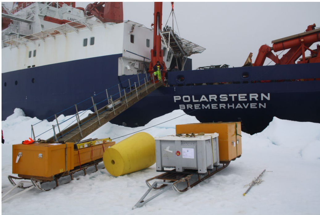
The ITP deployment apparatus was lowered onto the ice using the ship's crane and hauled to deployment site using sleds. (Raquel Somavilla)
