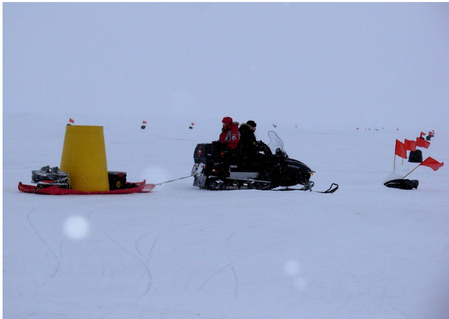
Using the snow machine to haul the ITP foam and wire rope reel to the deployment site. (Rick Krishfield)
