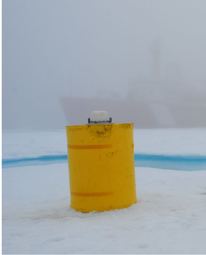
Shortly after installation, the foam flotation collar of newly deployed ITP 55 still shows the marks from its previous deployments as ITPs 4 and 24. (Mary-Louise Timmermans)
