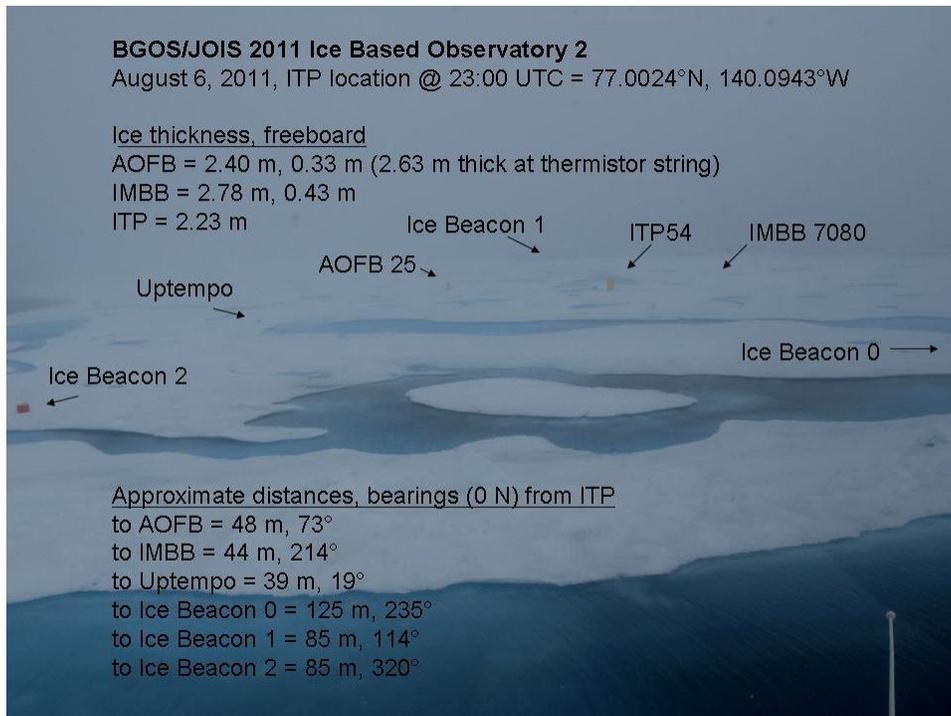
The distribution of the buoys on the floe, ice thickness and freeboard measurements at the buoy sites of the second IBO deployed during JOIS 2011. (Rick Krishfield)
