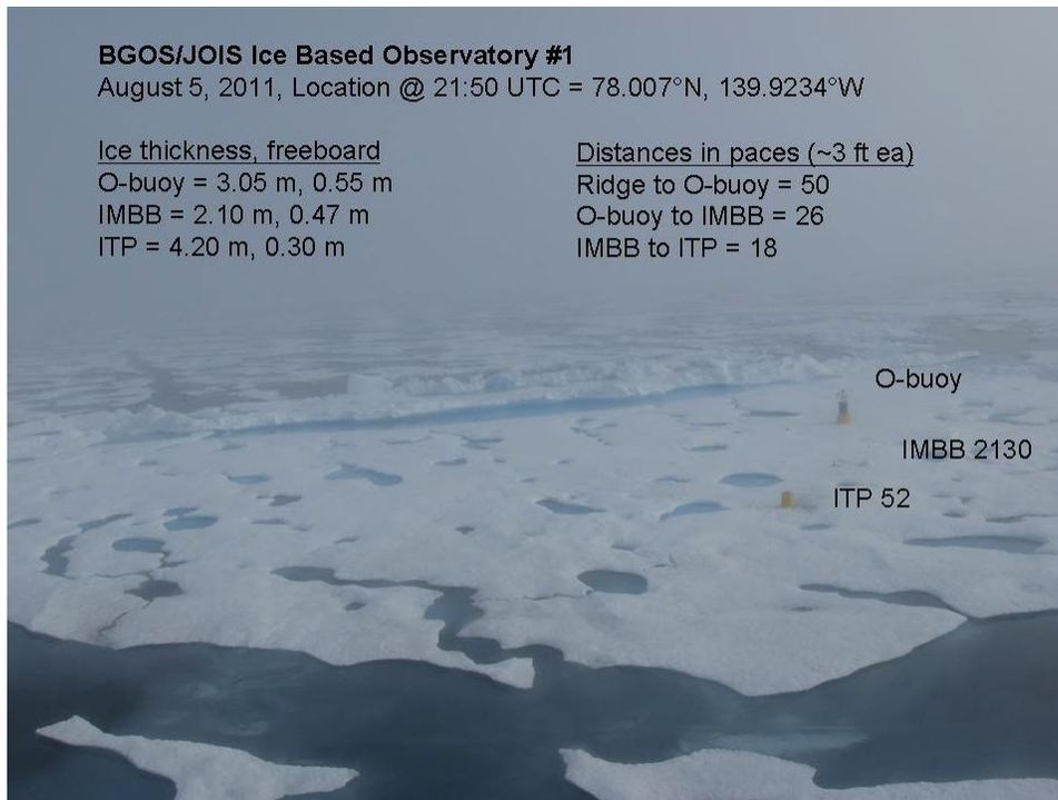
View from the last helicopter flight of the first IBO deployed during the JOIS 2011 expedition showing distribution of the buoys on the floe, ice thickness and freeboard measurements at the buoy sites. (Rick Krishfield)
