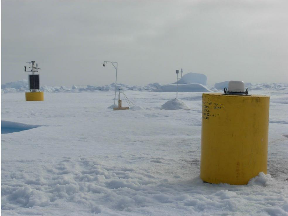
First Ice-Based Observatory deployed during the JOIS 2011 cruise consisted of O-buoy 5, IMB 2011-I and ITP 52 with biosuite package. (Rick Krishfield)
