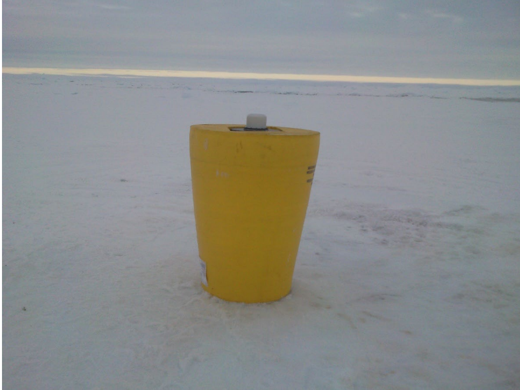
Surface package of ITP 49 shortly after the deployment during the 2011 TransArc expedition on the Polarstern. (Ben Rabe)
