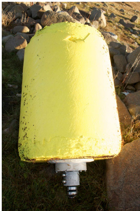
No tether, only surface package remained from ITP 47 when it was found onshore at Blacksod Bay in western Ireland nearly 2.5 years after installation. (Fergus Sweeney)
