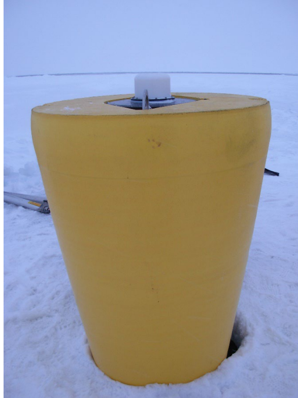
ITP 44 surface package effectively corks the 2 foot diameter hole in the ice required for the deployment of the MAVS profiler. (Rick Krishfield)
