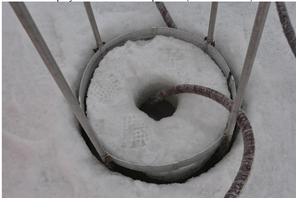
Water is supplied to the hot drill through the augered 4" diameter hole in the center. After the core is drilled, the 4" hole is also used to pass a toggle under the ice to lift the core for removal. (Kazu Tateyama)
