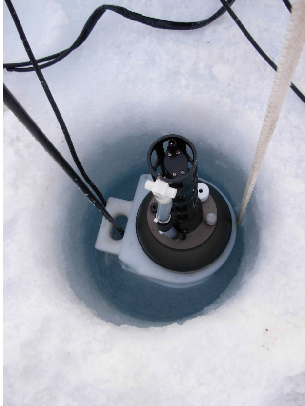
The ITP profiler was designed to just fit through the 10.5" diameter hole. (Rick Krishfield)
