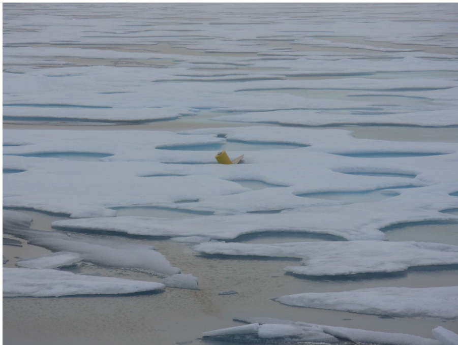
The surface buoy for ITP 4 is only partially submersed in the melt pond when it is relocated nearly a year after the deployment.
