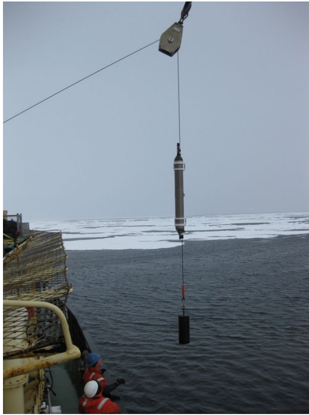
The ITP profiler sits on the bottom bumper during the over-the-side deployment.
