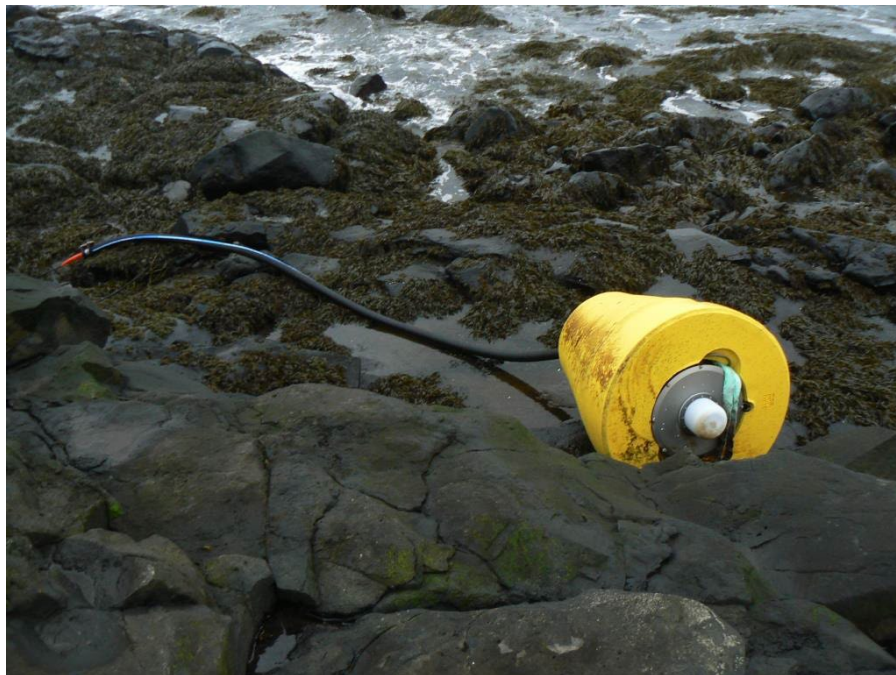
Two and one half years after deployment, ITP 36 surface package and partial tether was found washed up on the northern shore of Iceland. Additional data was eventually retrieved from the flash card memory of the surface controller. (Marvin Ingolfsson)
