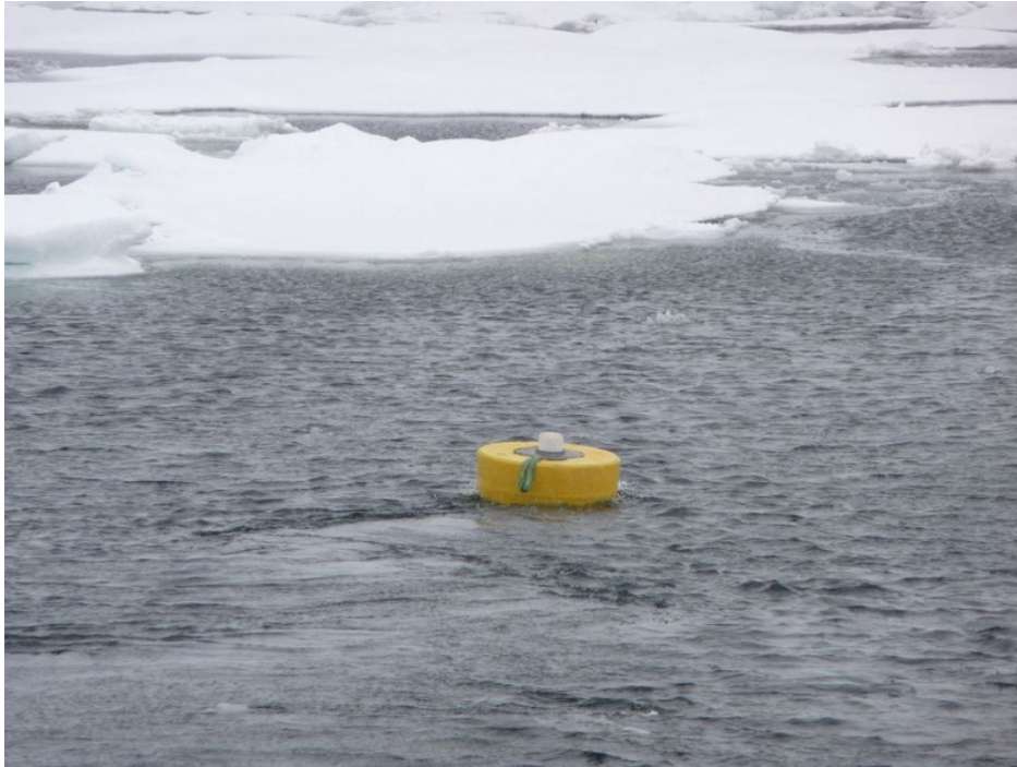
The first ITP deployed in open water sits about 25 cm above the waterline with the 790 m profiler mooring suspended below. (Jeff Pietro)
