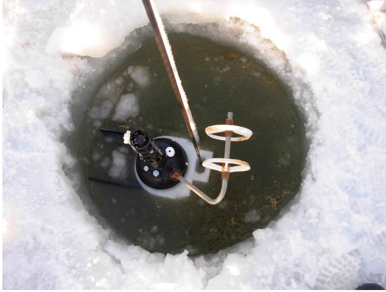
The ITP-V profiler is lowered into the 24" diameter hole to keep warm while the test of the inductive modem circuitry is performed. (Rick Krishfield)
