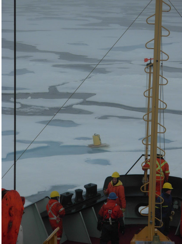
The Louis bears down on the re-righted ITP 33 in order to break up the icefloe containing the system. (Rick Krishfield)
