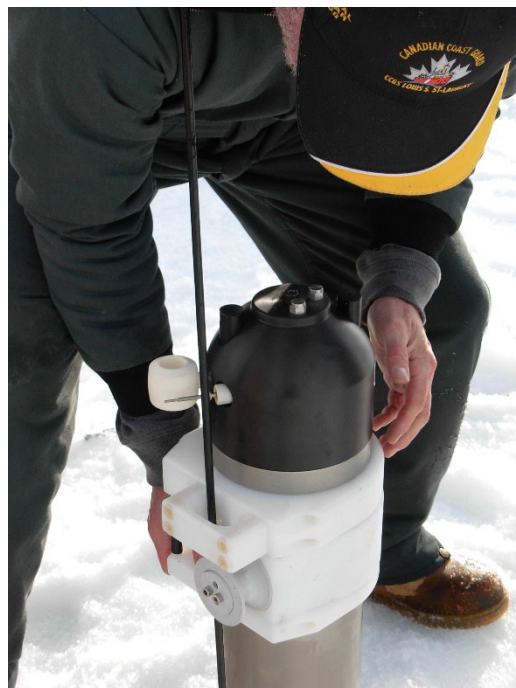
On this particular prototype ITP, the CTD sensors manufactured by FSI protrude from the side of the endcap, with the expectation that the wake effects of the instrument would be less. Here Rick Krishfield is lowering the package through the hole in the ice floe. (Photo by Gary Morgan)
