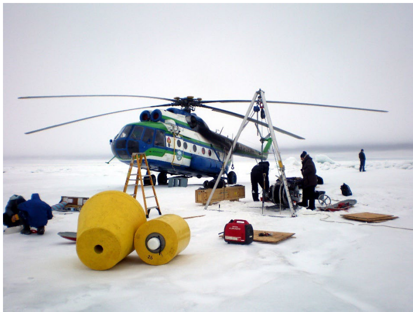
Once the tripod and other deployment apparatus were assembled, the ITP wire with 250 lb anchor were deployed through the 11" augered hole in the ice. It took approximately 30-35 minutes for the 790 m of wire to be deployed. (Photo by Sergey Unovidov)
