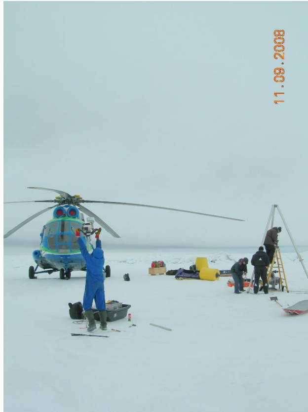
A Russian scientist stretches to auger a survey hole in the ice floe while the Sergey Unovidov assist Newhall and Pietro with assembling the ITP deployment apparatus.
