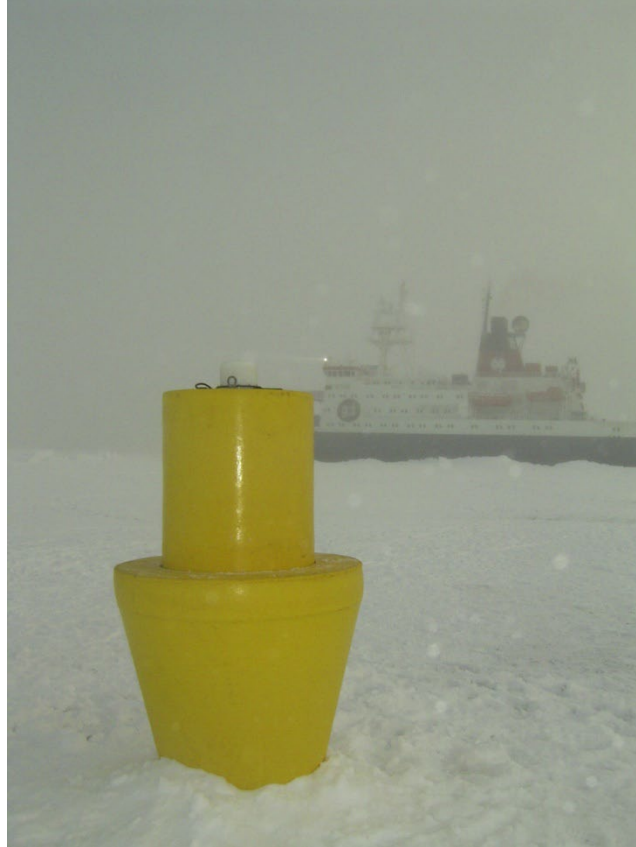
ITP25 surface package (with supplemental conical foam flotation) after deployment, with the Polarstern in the background. (Photo by Ben Rabe)
