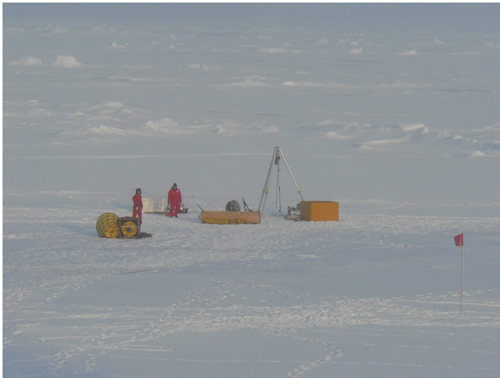
ITP 25 was deployed on a 1.5 m floe about 20 m from the ridge shown in rear. All of the gear was transported to the deployment site by helicopter.
