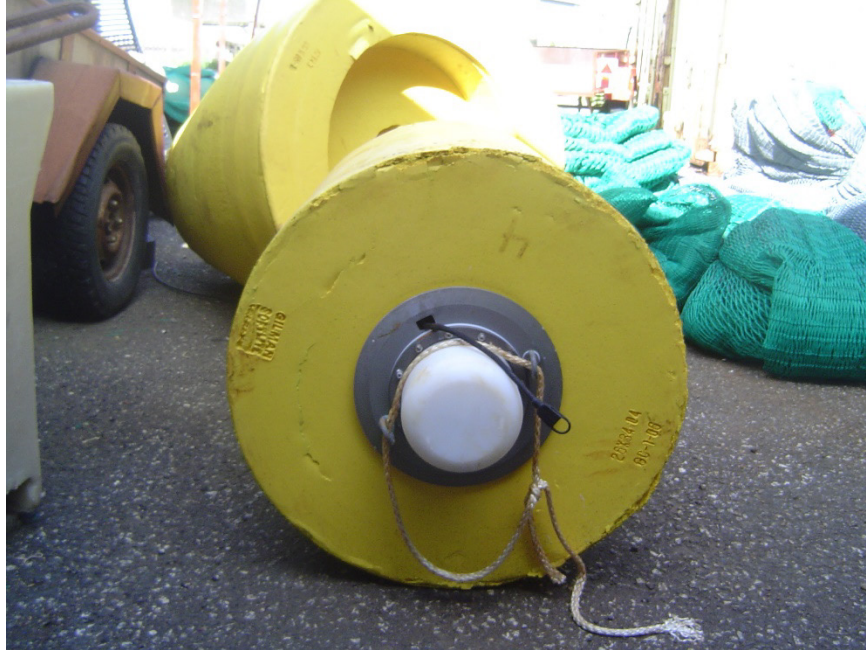
Two years after being deployed north of the Laptev Sea in the Eurasian Basin of the Arctic Ocean, ITP 24 surface package, supplementary foam and a portion of the tether was found floating in the Greenland Sea and recovered by an Icelandic fishing vessel. (Photo by Marvin Ingolfsson)
