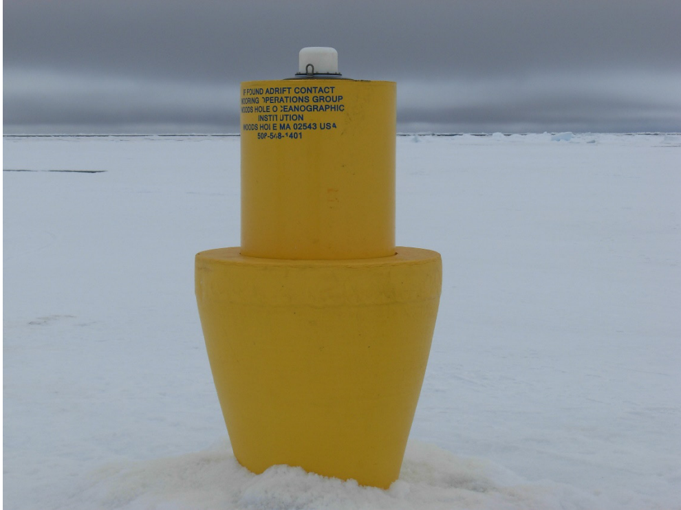
Surface package and supplemental flotation of ITP 23 after deployment near 82° N in the Beaufort Gyre. (Photo by Rick Krishfield)
