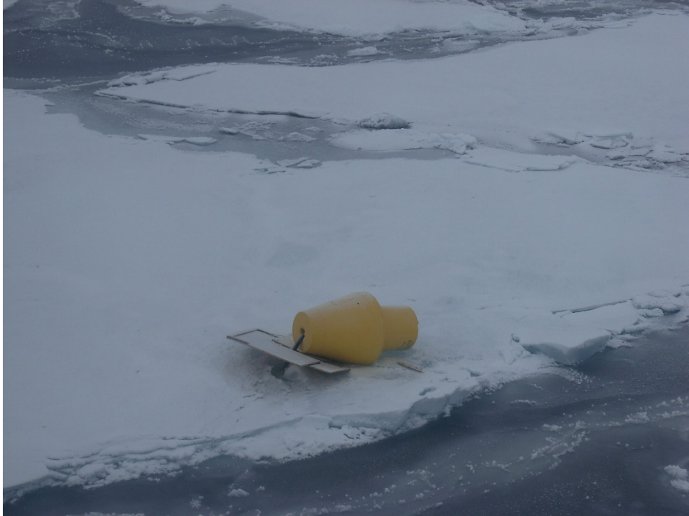
A little over a year after deployment, ITP 21 is found laying sideways on the ice because the cable is still frozen into the floe. (Photo by Rick Krishfield)
