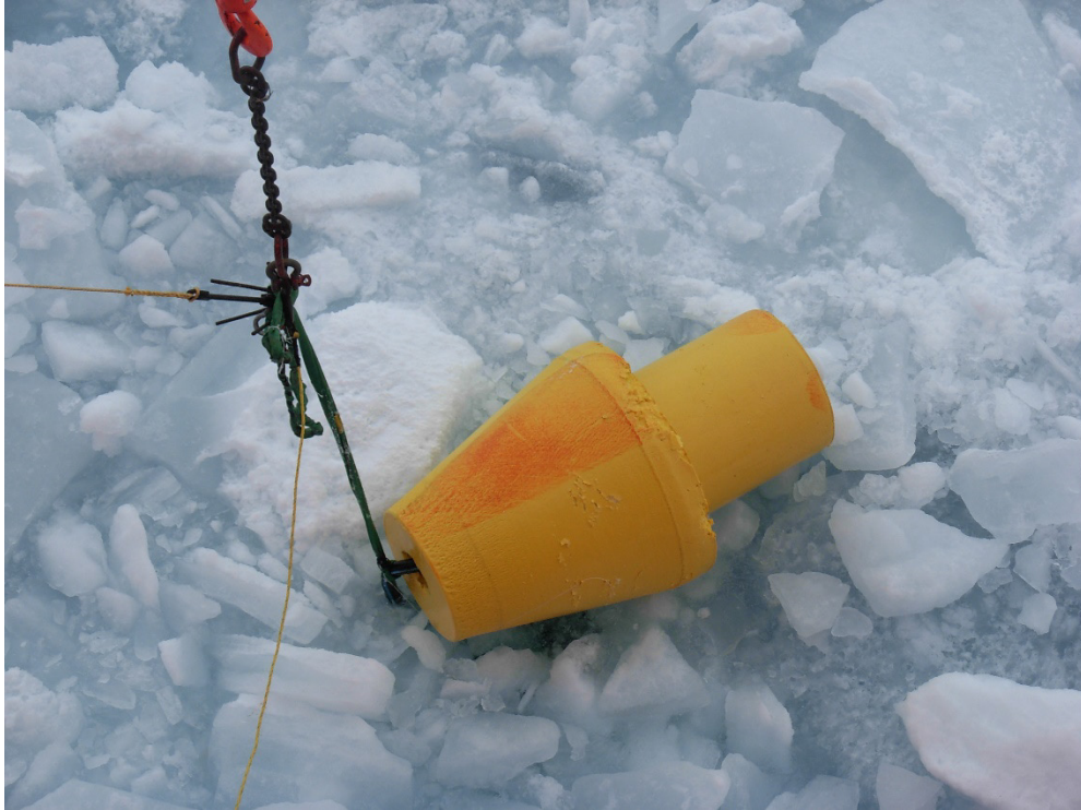
Grappled and hooked to the ship's crane, the ITP is ready to be hauled up on the sling. (Photo by Rick Krishfield)
