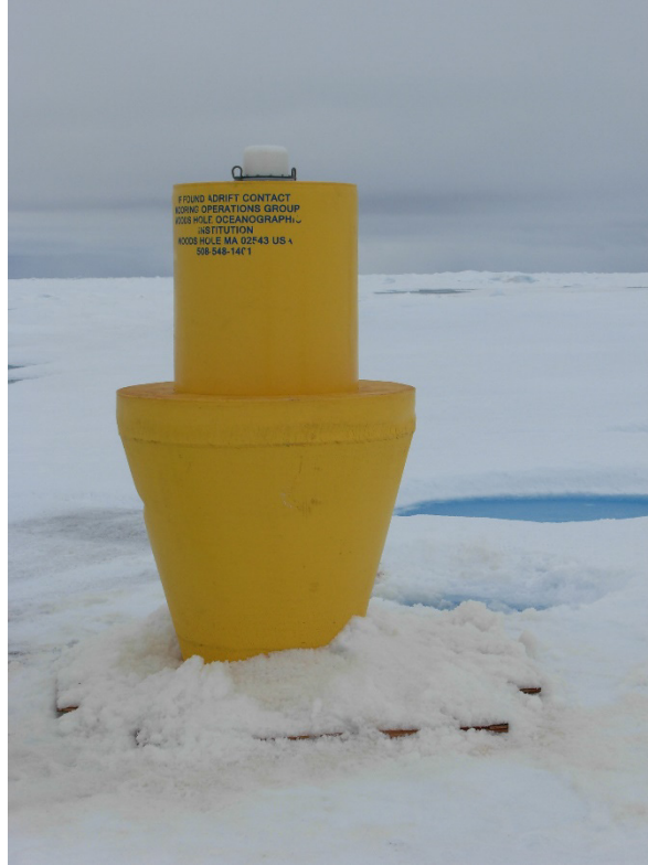
ITP 21 (and all ITPs deployed in summer 2008) included a supplemental conical flotation collar added to the standard ITP buoy in order to bring the surface electronics higher above the ice (in the event of ridging) and hopefully prolong the lifetime of the systems in less robust ice conditions. (Photo by Rick Krishfield)
