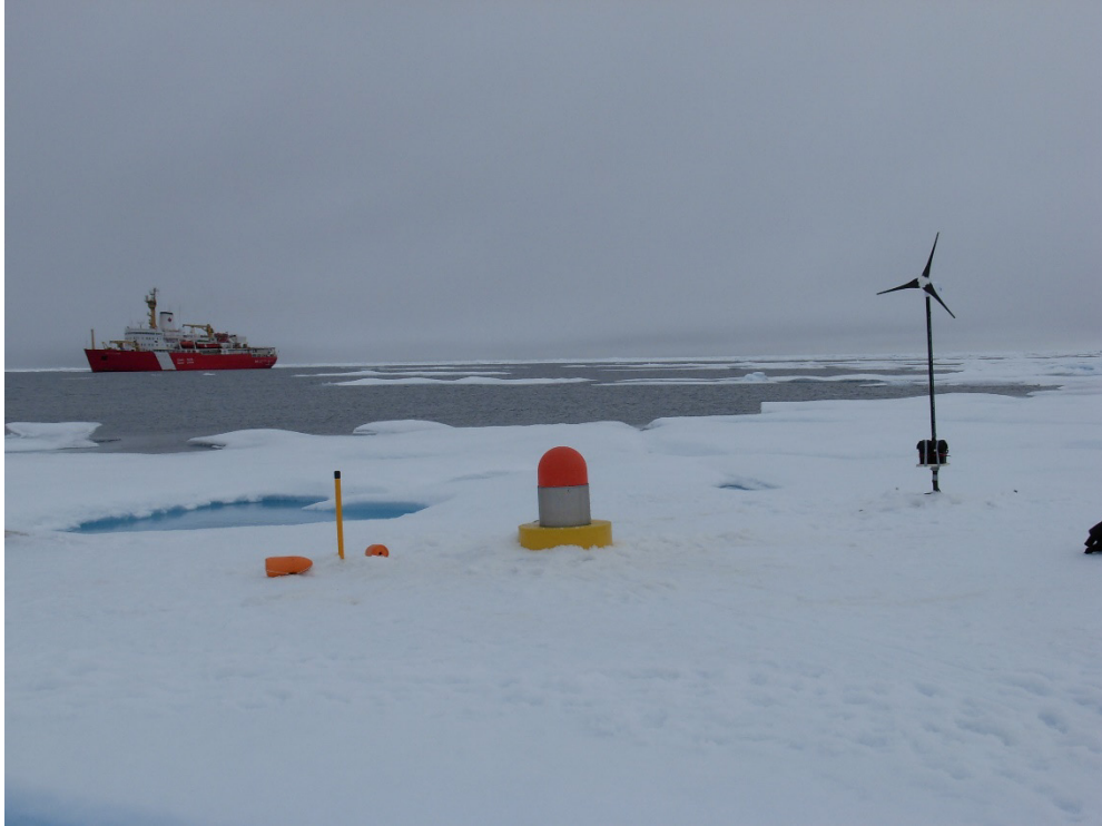
The AOFB is the first instrument installed, and the deployment apparatus is immediately moved to the ITP deployment site. (Photo by Rick Krishfield)
