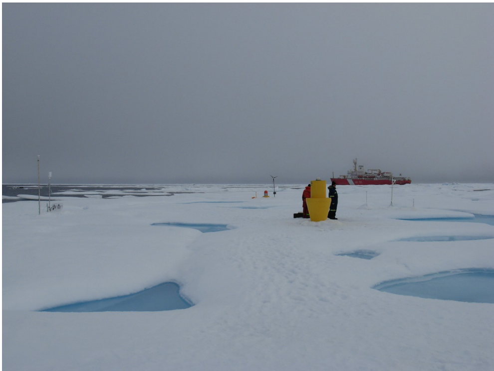
The ice based observatory consisting of SIMBA (left), AOFB (far), ITP 20 (near), and IMB (right) was deployed on a seemingly robust >3m thick ice floe. (Photo by Rick Krishfield)
