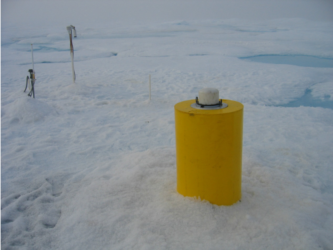
The combination of the ITP and IMB is an example of an Ice-Based Observatory (IBO) for obtaining sustained measurements of the atmosphere-ice-ocean in all seasons as part of the Arctic Observing Network (AON). (Photo by Rick Krishfield)
