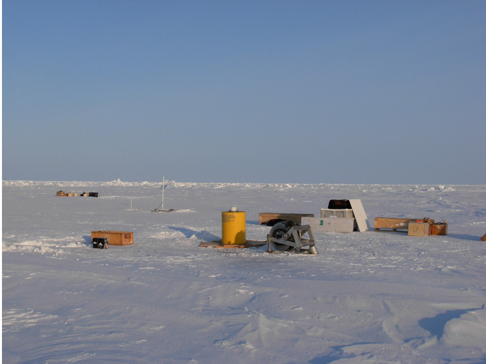
ITP 19 surface package is positioned on a pallet after deployment with the IMB in the background. (Photo by Rick Krishfield)
