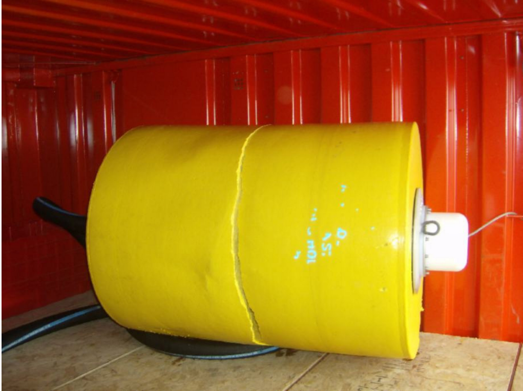
ITP 15 surface package after recovery by the CCGS Des Groseilliers in Baffin Bay three years after being deployed in the Arctic Basin. Note the crack that circumscribes the middle of the foam which was likely caused by ice ridging or compression amongst the bergy bits. (Photo courtesy of Brent Cauthier)
