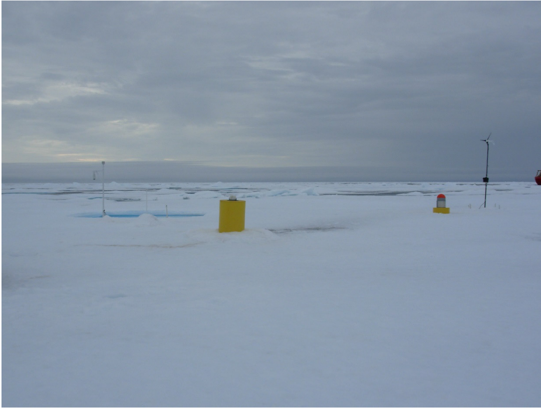
An Ice-Based Observatory consisting of an Ice-Mass Balance Buoy, Ice-Tethered Profiler, and Arctic Ocean Flux Buoy shortly after deployment in August 2007. (Rick Krishfield)
