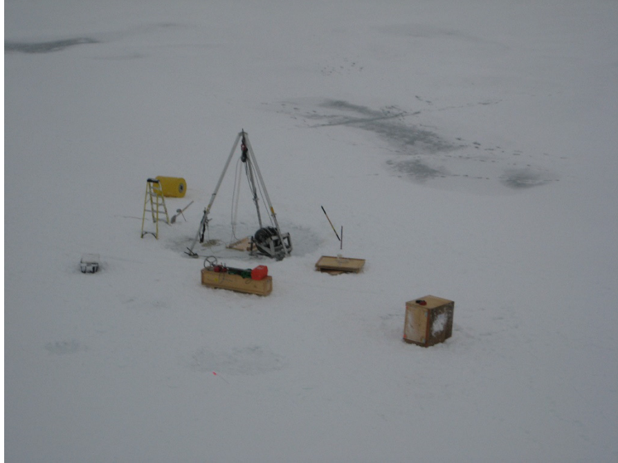
Aerial photo of the ITP deployment site after drilling the 11" diameter hole, but before deploying the instrument. (Photo by Ben Rabe)
