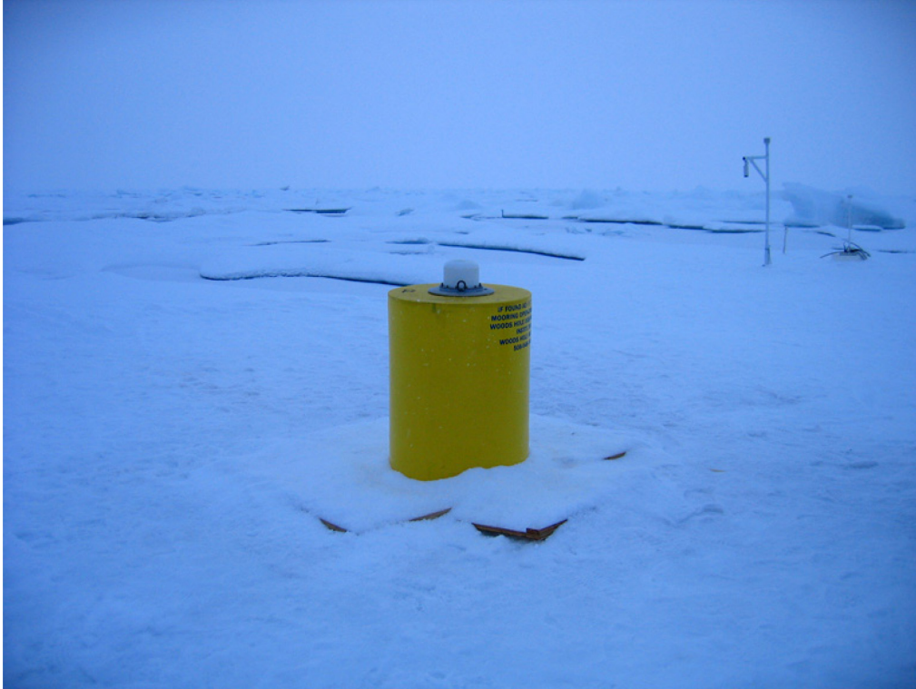
The first Ice-Based Observatory deployed from the Russian research vessel "Akademik Federov" in September 2007 consisted of ITP 11 and IMB on a 2.8 m thick icefloe. (Photo by John Kemp)
