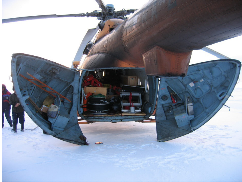
After landing on the selected deployment icefloe, the cargo bay doors of the Russian MI-8 helicopter are opened to unload the ITP instrument and deployment apparatus (and IMB). Photo by John Kemp.
